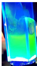
Figure 5. Greenish fluorescence light produced by the material in the violet light radiation
