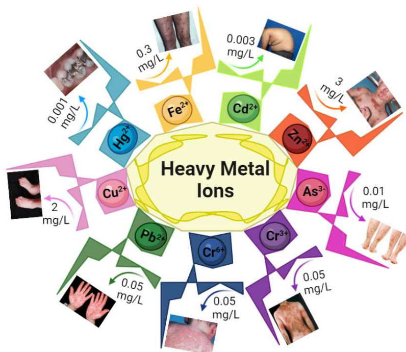
Figure 1. Effects of heavy metal ions in water and their effect on the human body, as well as their permissible values according to the standard of the World Health Organization.
