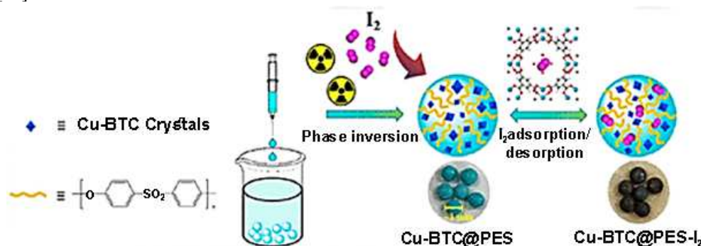
Figure 1. Millimeter-scale poly(ether sulfone) composite beads loaded with porous Cu-BTC [ \text{Cu}_3(\text{BTC})_2 ]. Reprinted with permission from ref [11].
