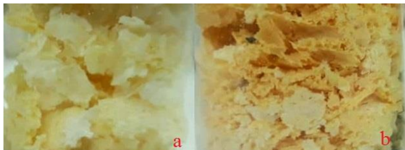
Figure 1. Synthesized PZT powders; a- pure PZT powder, and b-PZT:K powder.
